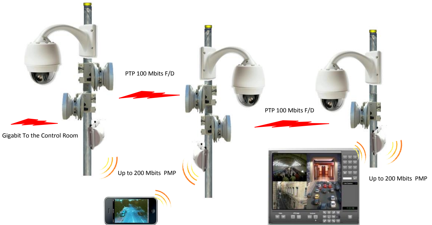
Along the Street, powered by the Light Mast, Hypercable Wi200S Autonomous CCTV with lithium-ion batteries. Backbone Ring Mesh and 3-4G Offload Acces Point 2.4 and 5.4 GHz design. F/D 1.000 or 100 Mbits
