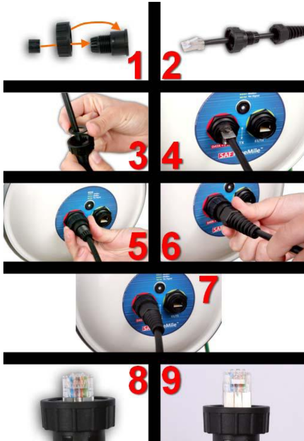
Figure 6. Assembling Ethernet weatherproof connector
