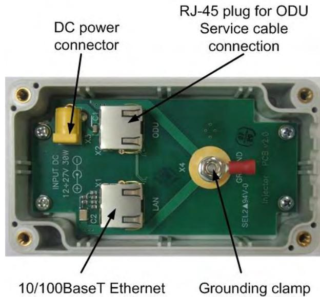
**Connection scheme for IDU-LA (for second Ethernet port)**
