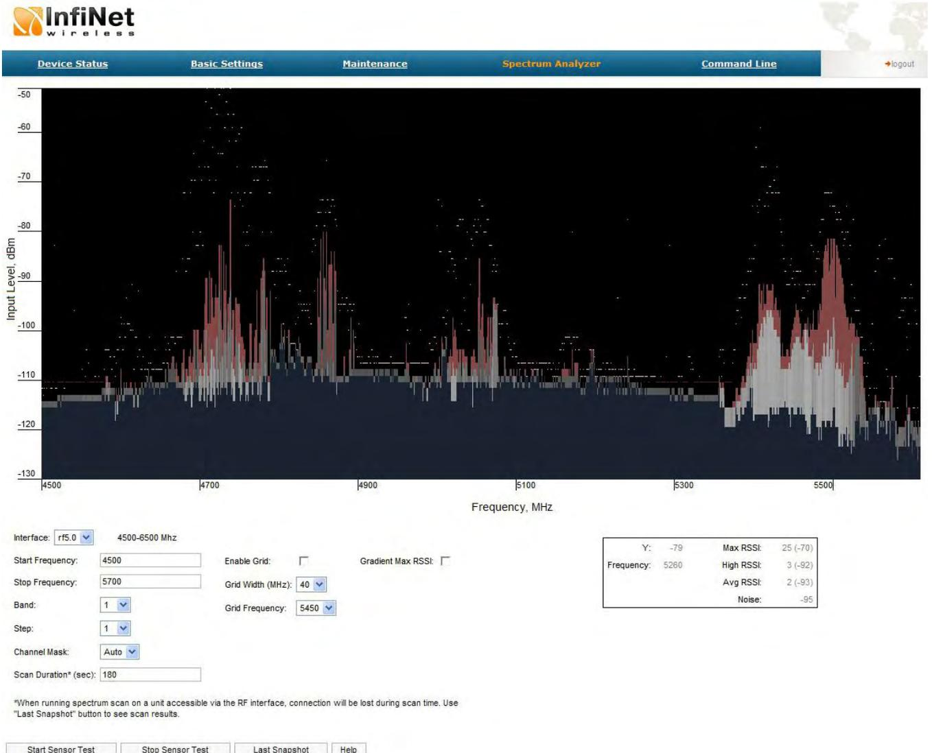
The «Spectrum Analyzer» page provides deep analysis of radio emission sources. In this mode device scans the radio spectrum on all available frequencies. To obtain information as complete as possible, the scanning process may take some time.
