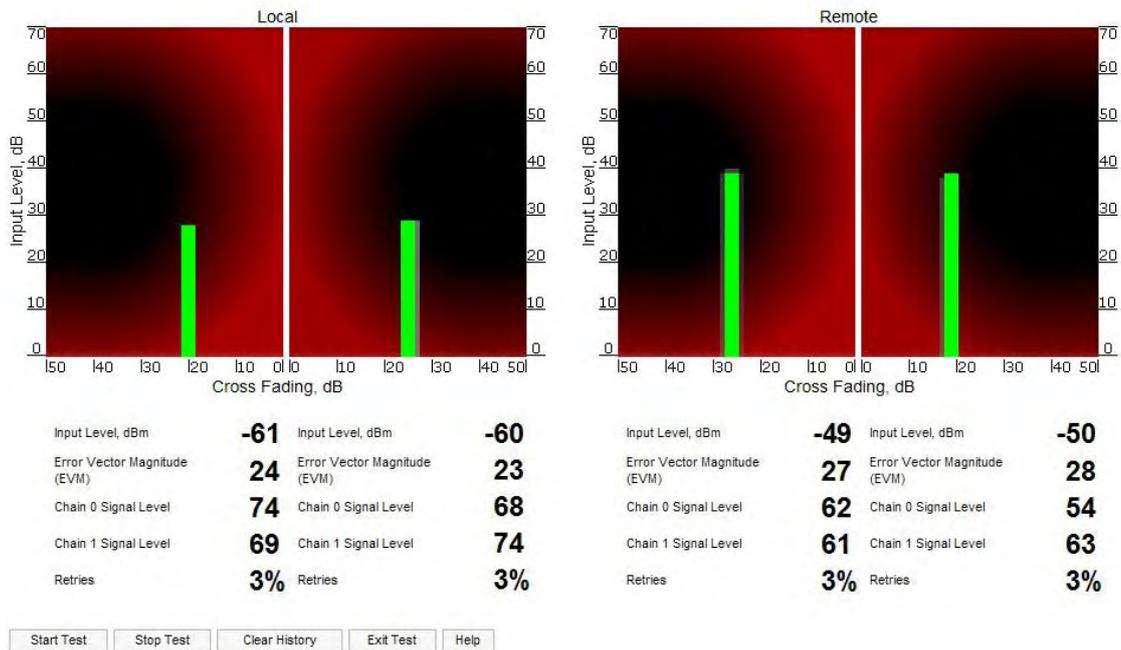
"Start Test"/"Stop Test" buttons at the bottom of the page start/stop the alignment test. "Exit Test" button returns to the "Device Status" page. "Help" button displays help guidelines for antenna alignment.
