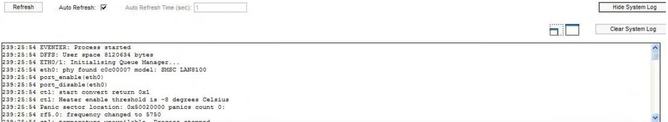
The "System Log" section allows browsing the unit's system log. It is possible to minimize/enlarge the system log window with the following buttons:
