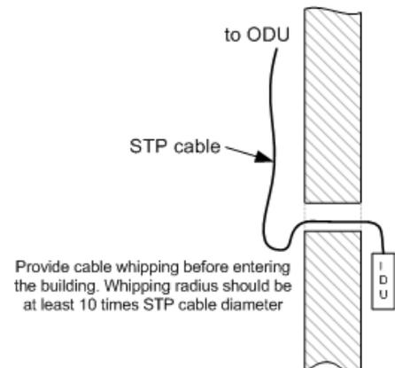
**⚠ It is extremely important to install ODU connectors down!**
