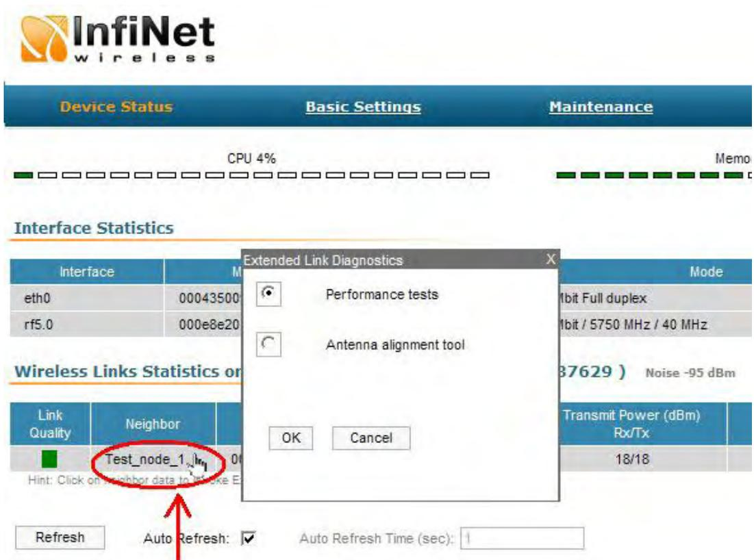
Then choose "Antenna alignment tool" or "Performance tests" from the appeared "Extended Link Diagnostic" window.
