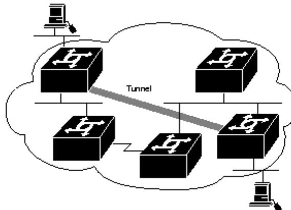
There are several approaches to build tunnels. One of these, IP into IP Encapsulation (described in RFC 2003), is implemented in OS WANFlex. This technology is used, for example, in Cisco Systems routers, and is a subset of the IPSEC protocol supported by several operating systems.
