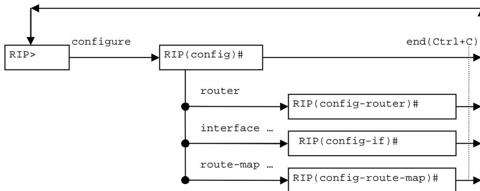
One can set the necessary mode or execute commands without specially entering into arip module. For example, if we consistently execute the following commands:
