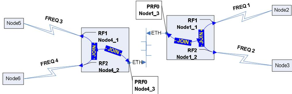
In this example we have joined several distributed (possibly even geographically distributed) network segments. Combining “joins” for different radio interfaces and pseudo radio interfaces the network will obtain a good number of alternative paths in any direction thus providing with the best delivery quality and less bottlenecks.
