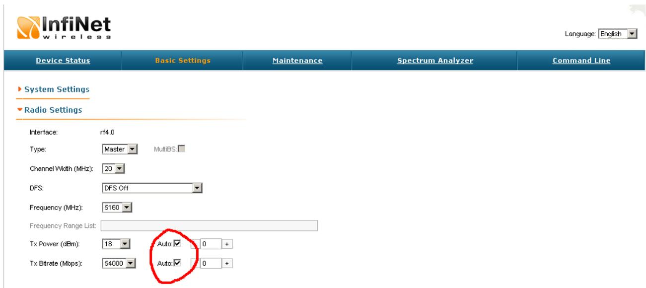
Figure 3. Radio settings configuration section
