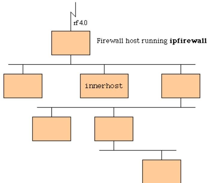
All subnets of an inner network, including a host address innerhost, are owned by the one network (or a network group). Let's imagine that outer network has no hosts which are within the range set up for the inner network. Therefore, all the packets that are accepted via rf5.0 interface of the router with firewall run on it and have the source address which is in the range of addresses of the inner network must be blocked. The following command can perform this action:
