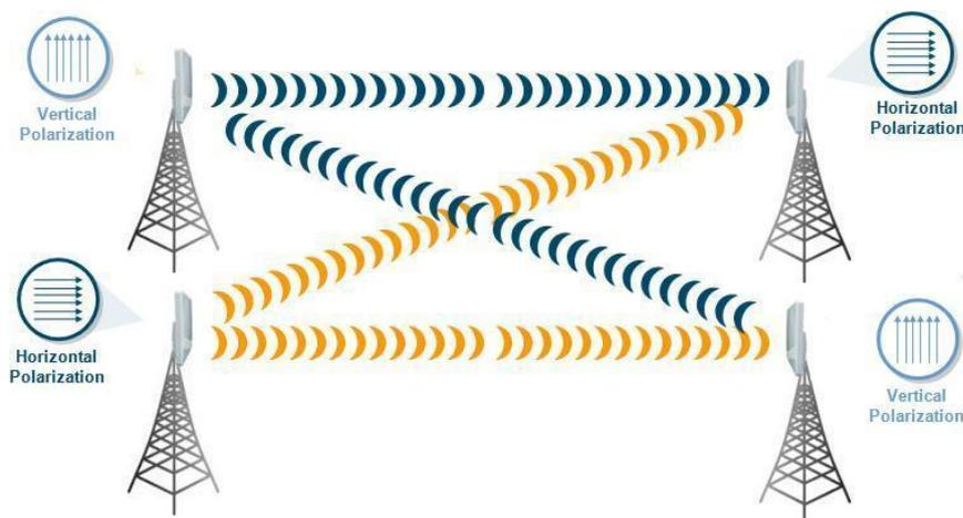
Figure 2. Data transmission path in InfiNet Wireless MIMO products in MISO mode
