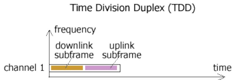
Classical TDD systems (Exalt, Orthogon) allow only fixed ratio for incoming/outgoing data flow (50:50, 30:60, etc.). Some systems (e.g. Winlink and most microwaves) allow fixed 50:50 ratio only without the capability to alter ratios. Other TDD systems can be statistically adjusted from the base ratios.
