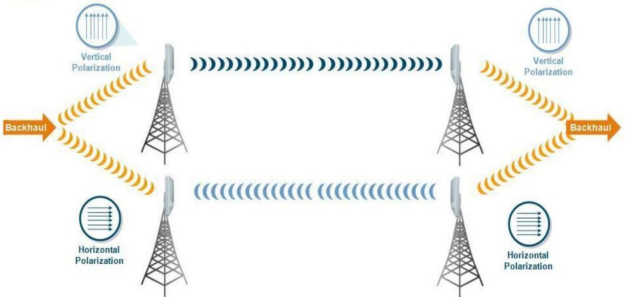
Figure 1. Data transmission path in InfiNet Wireless MIMO products
