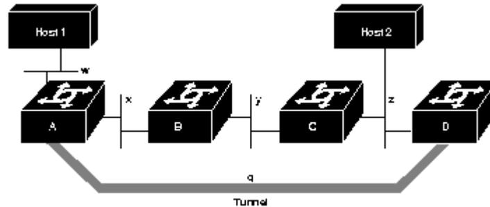
Tunnels also solve the problem of using common transport media in a public network so that different clients could be provided with services by several providers. It means that a client can be connected by a tunnel to a specific provider, to be serviced by that provider, irrespective of the client's connection point to a common transport network.
