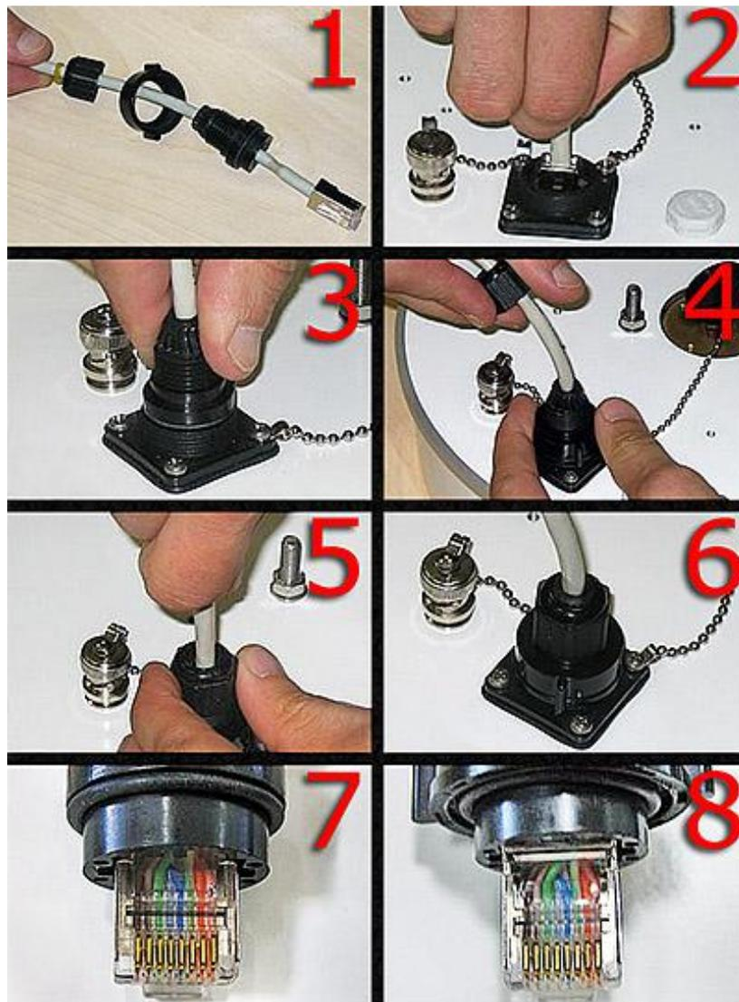
**Figure 2.1.** Assembling Ethernet weatherproof connector
