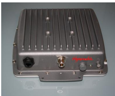
Modem Radio Full Duplex 200 Mbps
