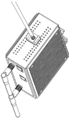
**STEP 1:** Screw the cable holder onto the bottom of the AWK-3131.
