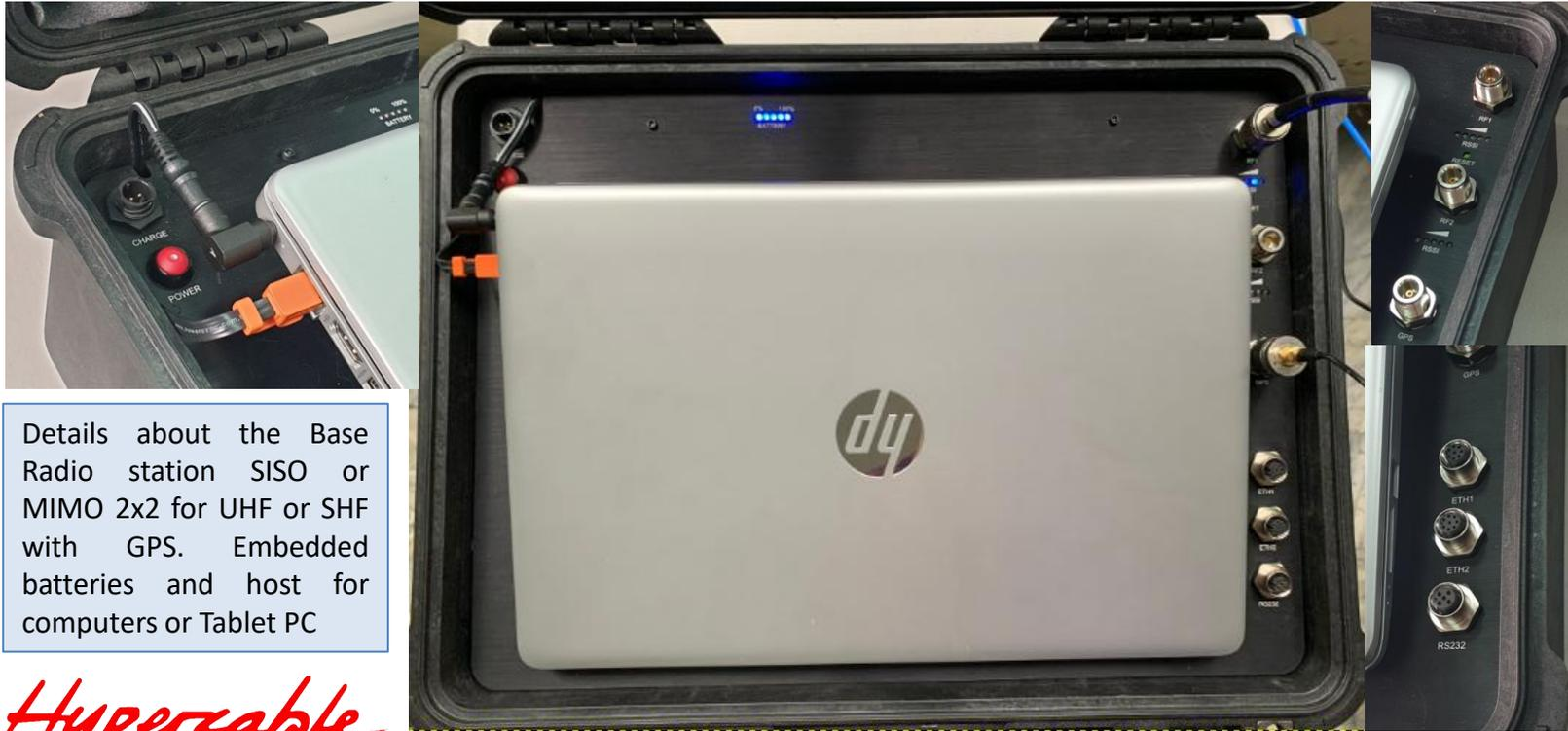
Details about the Base Radio station SISO or MIMO 2x2 for UHF or SHF with GPS. Embedded batteries and host for computers or Tablet PC
