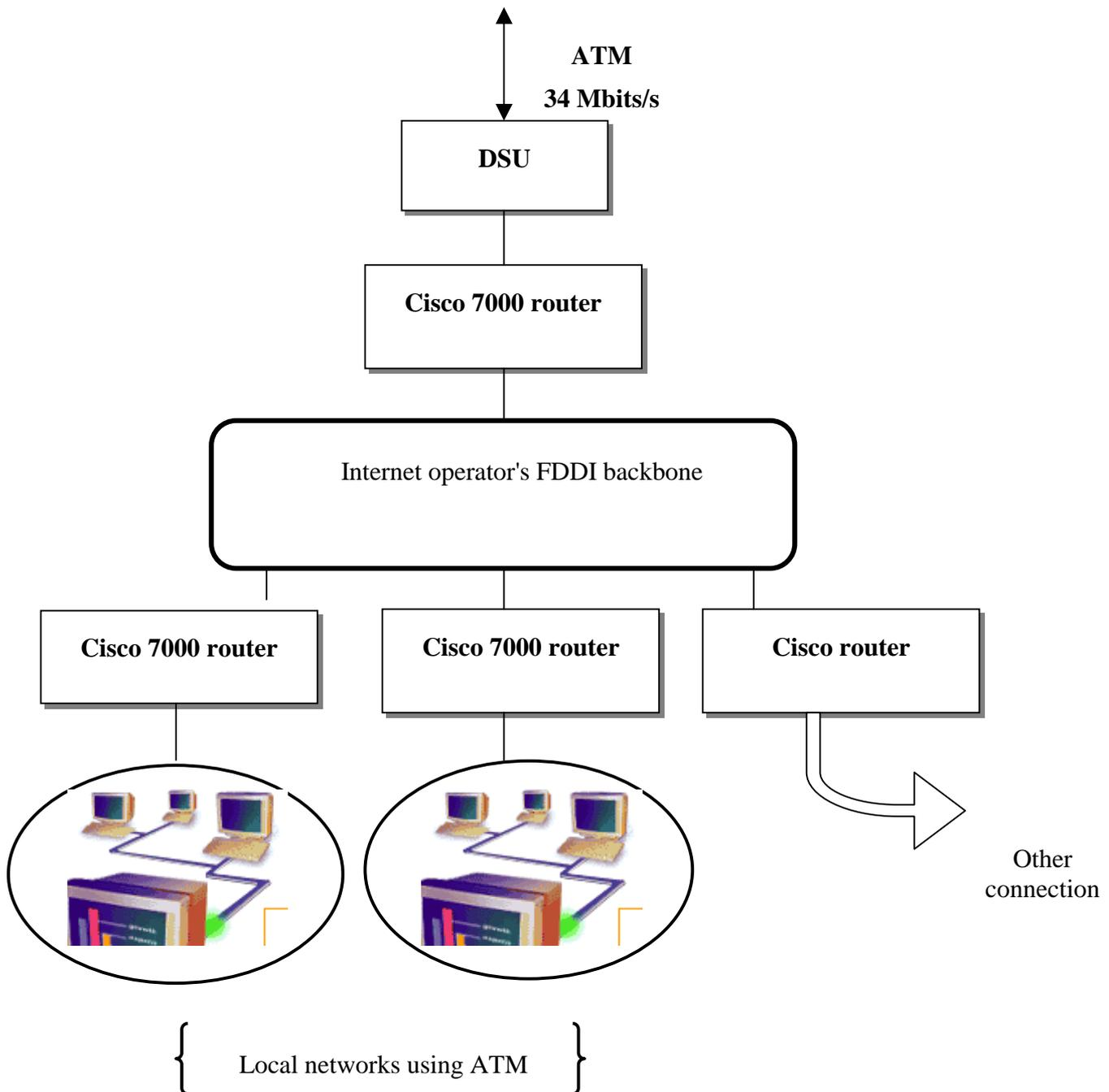
*Fig. 5.1 Outline diagram showing connection to ATM backbone*
