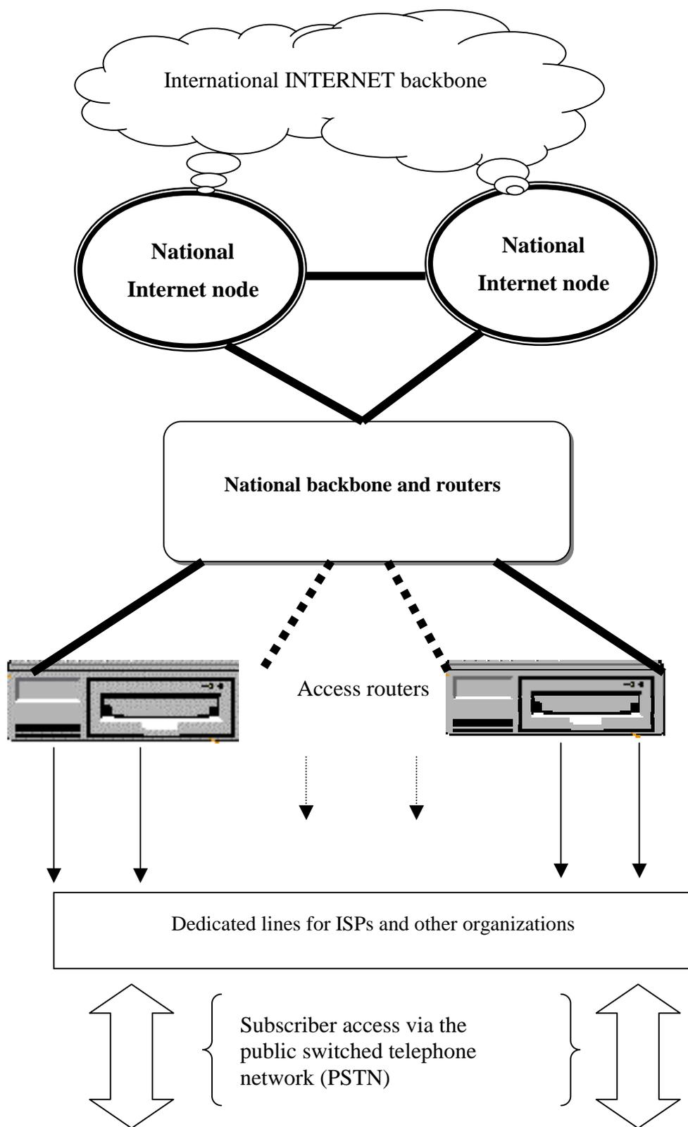
Fig. 3.8 Typical architecture of a network used by a national Internet services operator
