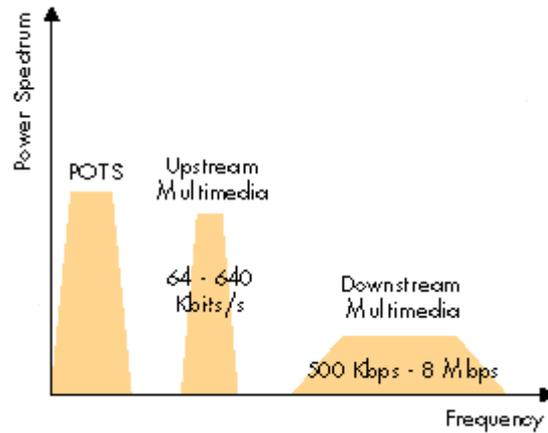
Fig. 5.3 The three ADSL communication channels
