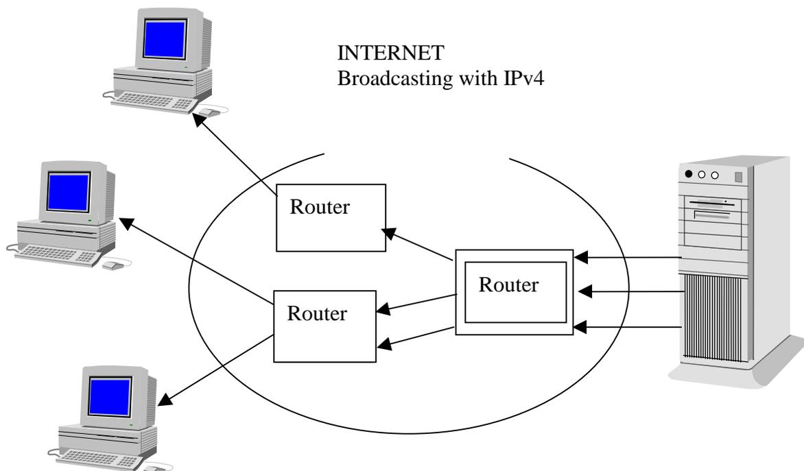
Fig. 2.3 Broadcasting with IPv4
