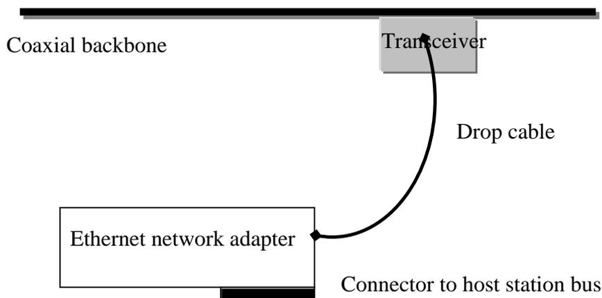
*Fig. 2.5 Main components of an Ethernet network*
