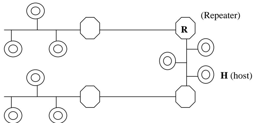
Fig. 2.6 Standard Ethernet configuration with maximum five segments
