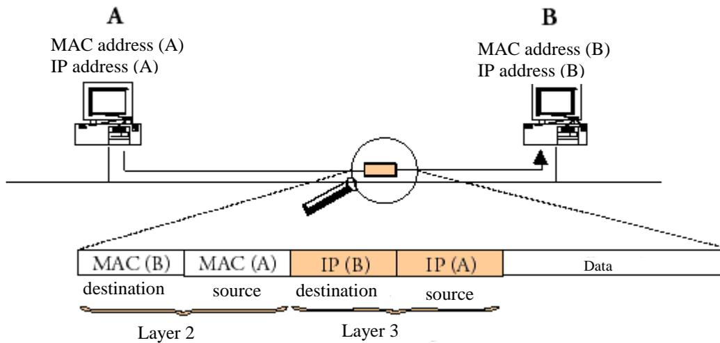
Fig. 3.4 Ethernet segment (Source: FI-6/1998)
