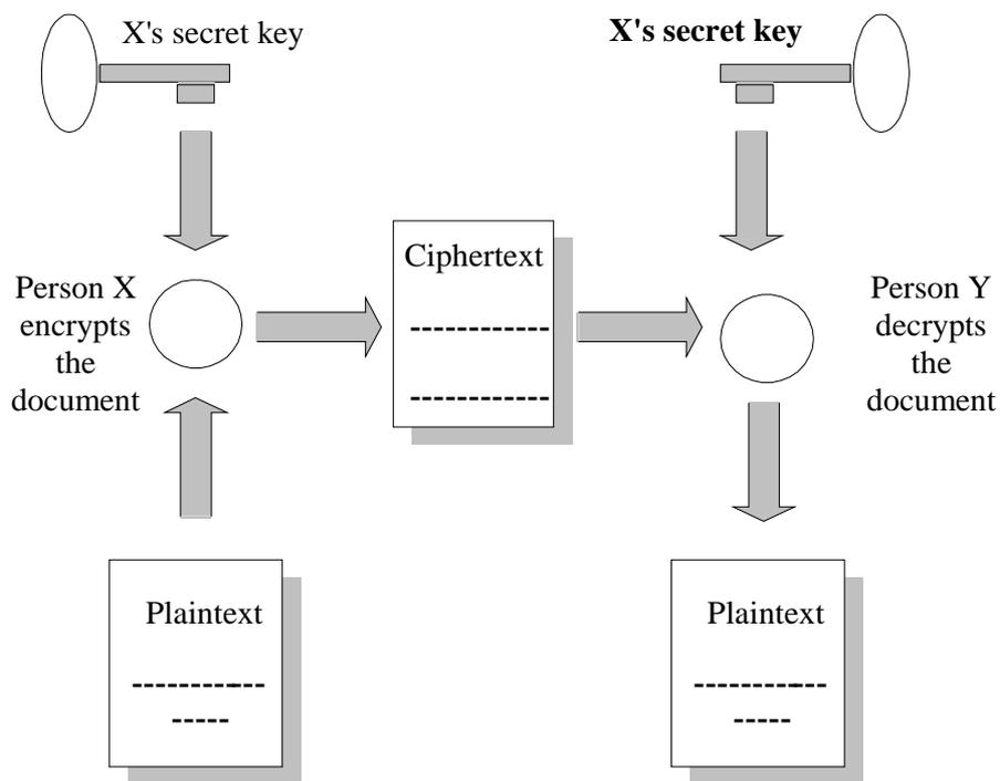
Fig. 3.11 Outline of encryption using symmetric algorithms
