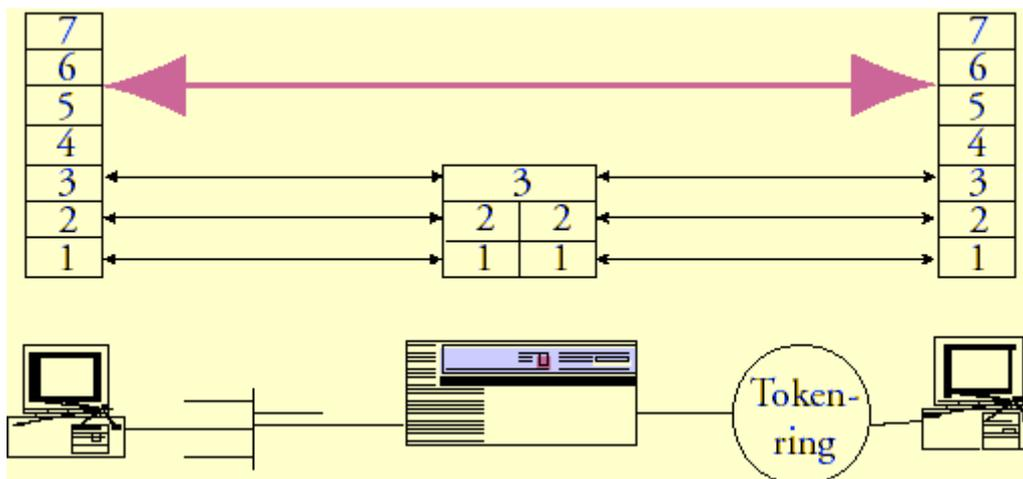
Fig. 3.1 The layers of the OSI model (Source: FI-6/1998)
