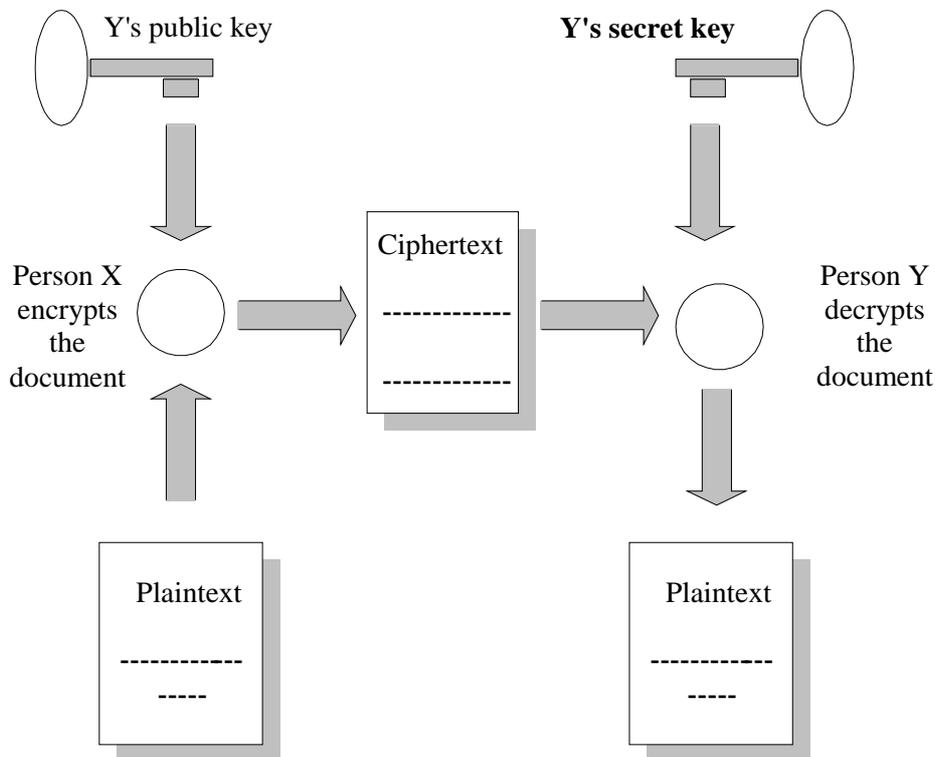
Fig. 3.12 Outline of encryption using asymmetric algorithms
