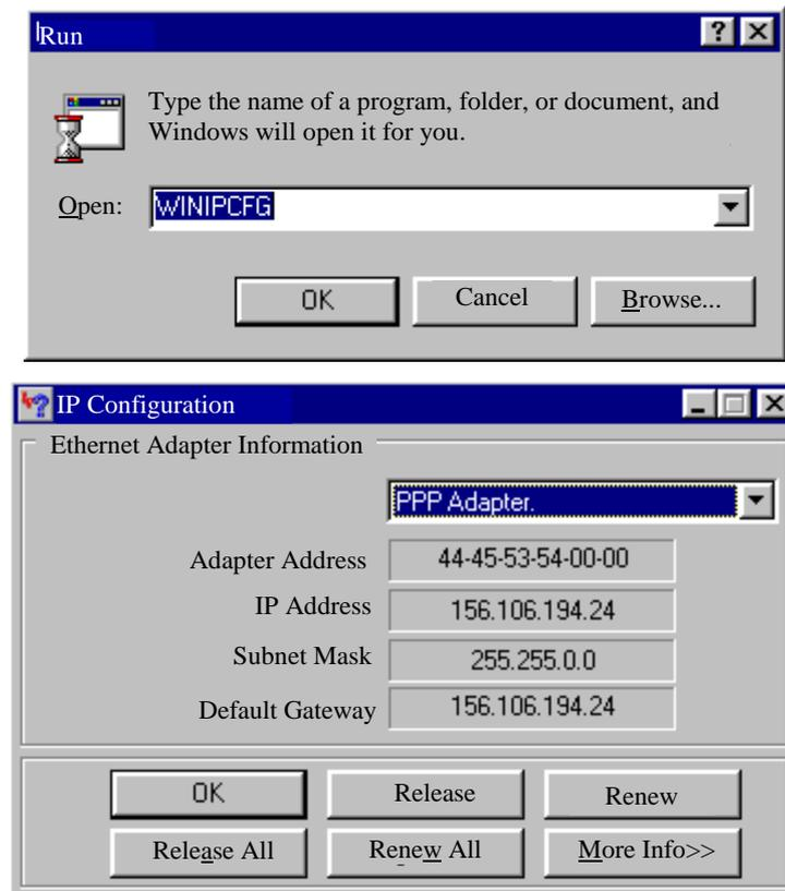
Fig 2.2 Checking the host's IP address on the network (ITU host)
