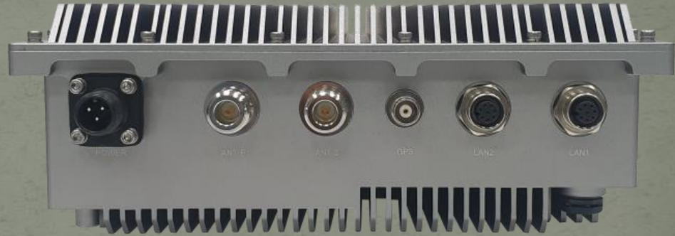
4.5 GHz 3 Watts MIMO Radio
