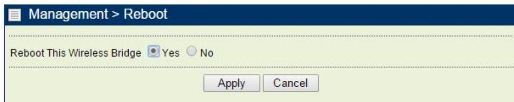
The Reboot screen enables you to reboot your 4GHz 2x2 MIMO Radio if any changes are made and you want to refresh the radio, you need to reboot the 4GHz 2x2 MIMO Radio. Select the “Yes” check box and click “Apply”. It will take you about 50 seconds to go through reboot. The Web-browser will not be accessible until the 4GHz 2x2 MIMO Radio has finished its reboot process.
